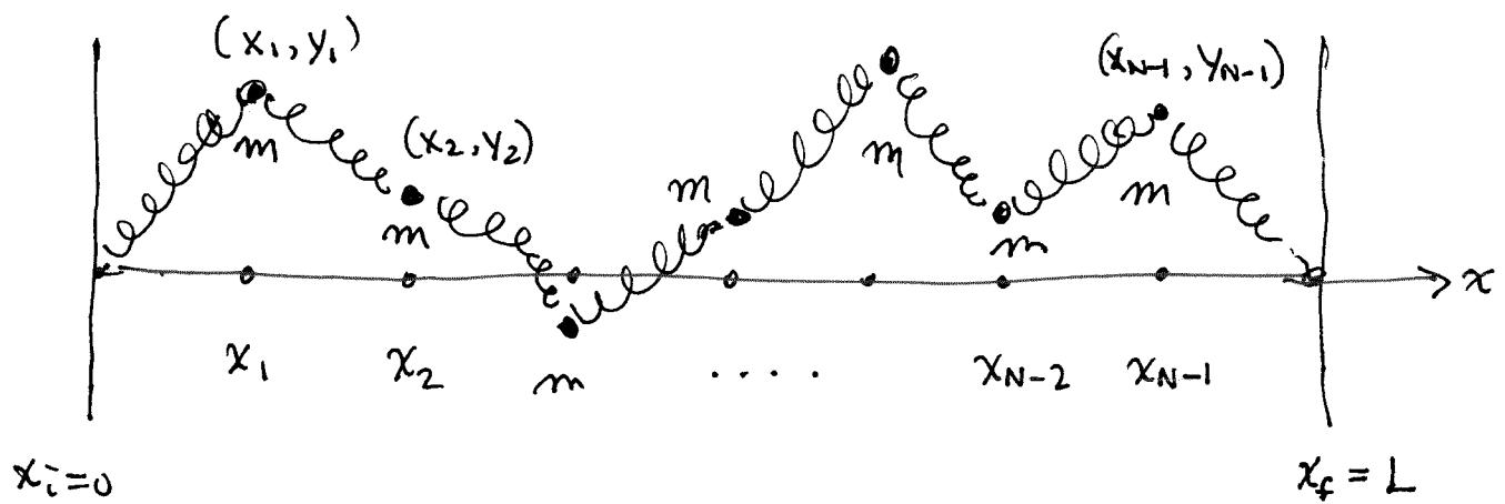
For simplicity we assume each mass is free to move only in the  $y$ -direction. This means that we are looking at only one transverse polarization or mode of oscillation. A real string could also move in the  $x$ - and  $z$ -directions. (The  $x$ -direction would be a longitudinal polarization.)
